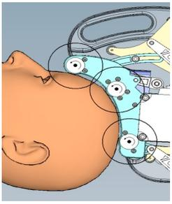
**Figure 1.** Diagram of sTMS device. Cross-sectional drawing of the arm of the sTMS device showing the location of the rotating magnets (indicated by cylinders with arrows) in relation to subjects' head.
